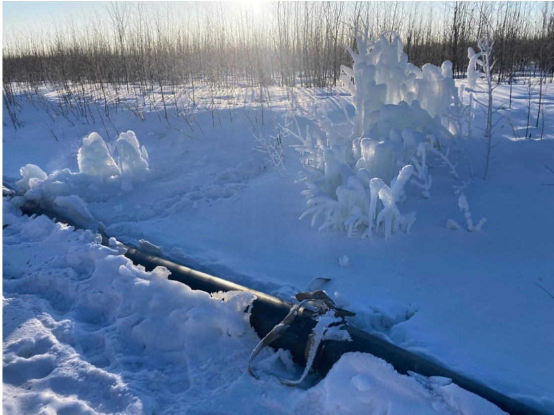
Figure 3. McGregor, David. 2025. Water Escaped from the Frack Line . Goodfare, Alberta.
